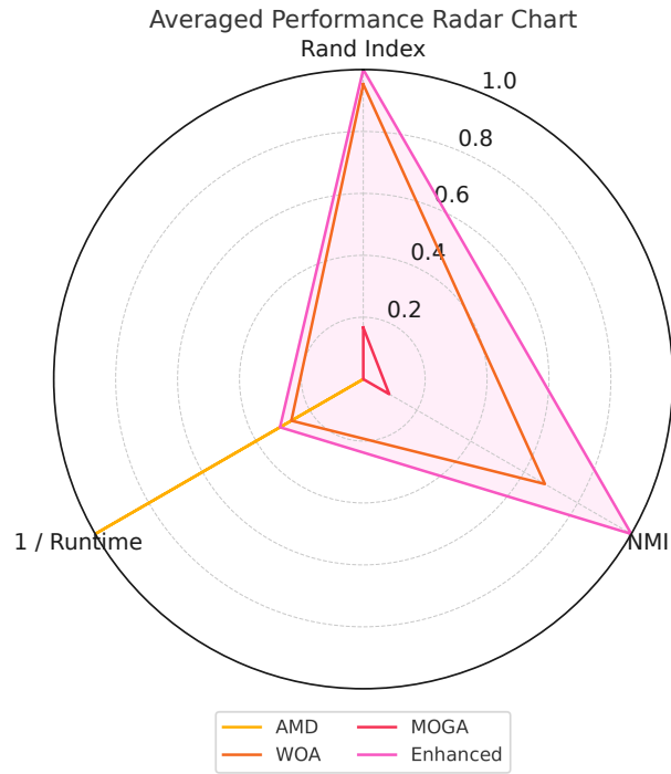
Figure 3: Normalized radar plot averaged across benchmarks. Enhanced MOGA-DBSCAN shows the most balanced and optimal performance across RI, NMI, and inverse runtime.
