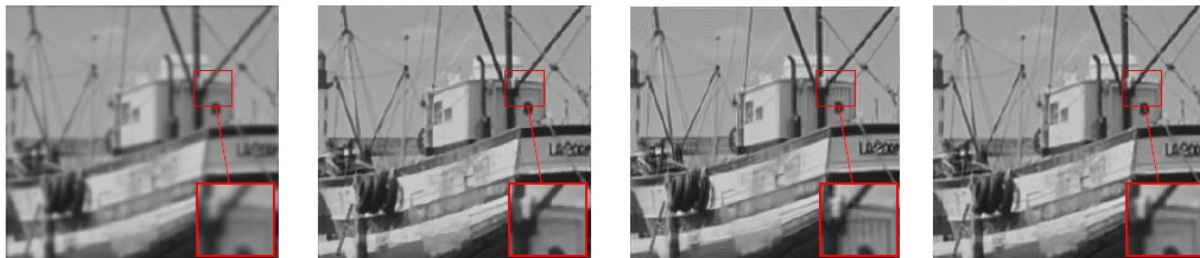
Figure 1: Visual comparison of image deblurring on gray image Boats ( 256 \times 256 ). From left to right and to bottom: original image, noisy and blurred image by Gaussian blur with the standard deviation of 1.6, the deblurred image by TVMM, BM3DDEB, and our proposed approach.
